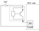
3-wire (PNP) proximity switch wiring
