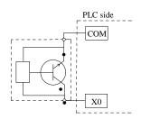
3-wire (NPN) proximity switch wiring
