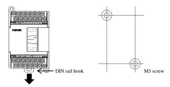
The PLC unit and expansion module are installed on DIN46277 rail (width 35mm); to remove, just pull down the assembly hook of DIN rail and take down the product.
