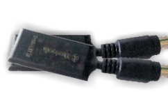
COM-BLUETOOTH (Bluetooth module, to realize wireless connection)
