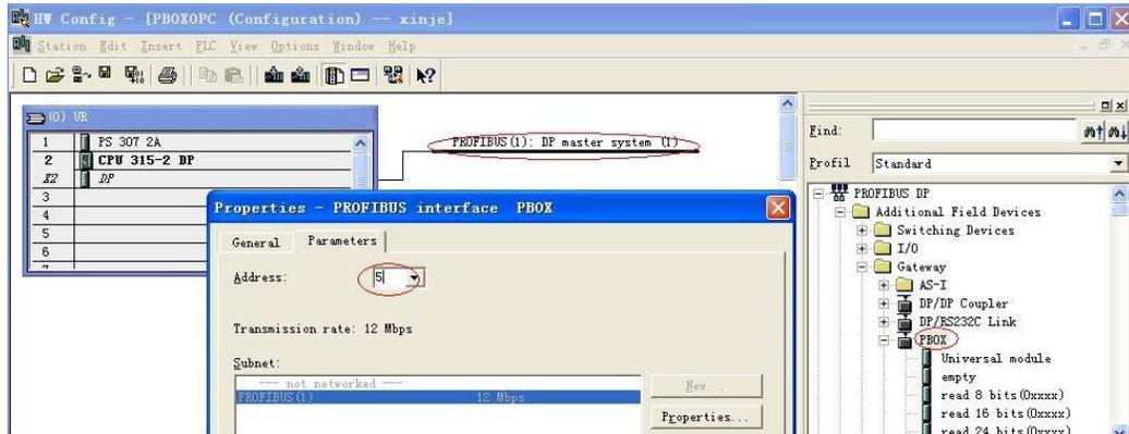
(14) As the chapter 1 said, we copy the file XC-PBOX.GSD to \.\Step7\S7data\gsd\, and copy the file Xinje\_B.bmp to \.\Step7\S7data\nsbmp\, now we can see the Xinje station picture in the below window:
