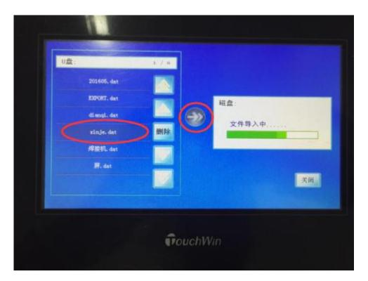
When the green process bar fulled, the import is completed. Please turn off the DIP switch 3, then restart the HMI.
