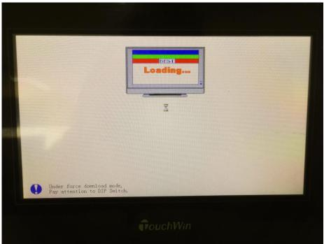
Wait for a moment, when it has "di di" sound, it means the import is completed. Now turn off the DIP switch 2, restart the HMI.
