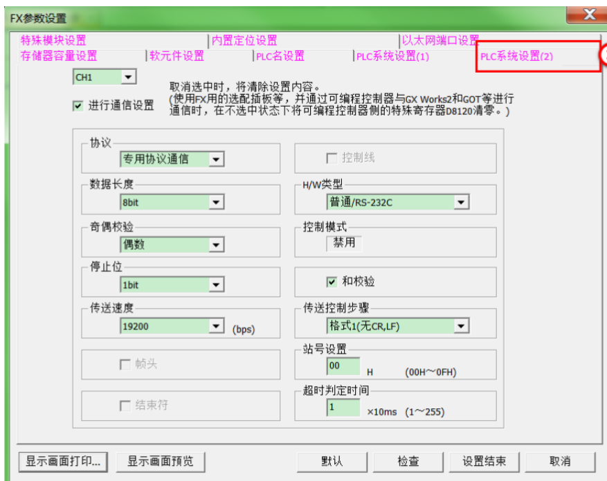
PLC left extended BD board setting
