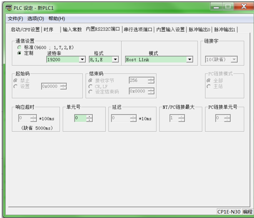
PLC serial port 1 settings
