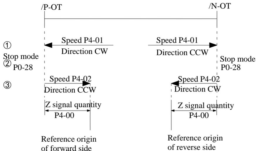
Sequential diagram of finding reference origin on forward side:
