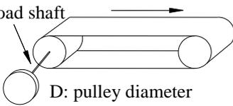
$1 \text{ rotate} = \frac{\pi D}{\text{command unit}}$      |
