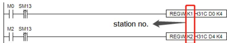
(2) Communication address: the address of the servo slave station. For the address of a register, please refer to Appendix 4. MODBUS address table.
