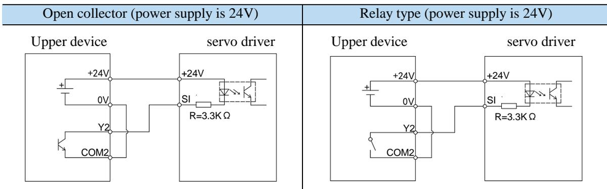
Note: SI5 terminal is high-speed input port, and SI1-SI4 are low-speed input ports.
