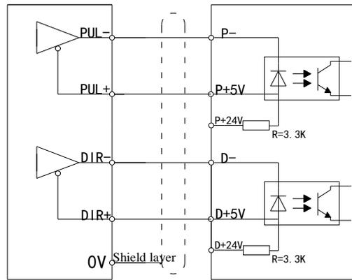
When the upper device uses 5V differential signal output, the graphic connection method is adopted, please pay attention to suspending P+ 24V and D+ 24V.
