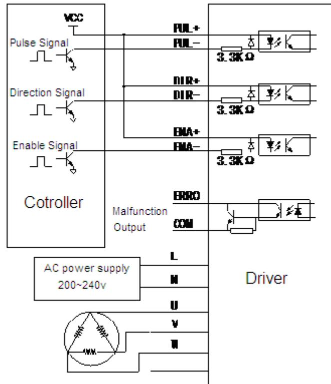
**Note:** Please separate the power cables (motor and power supply cables) and weak electricity cable (signal cables) to avoid interference.
