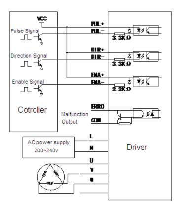
**Note:** Please separate the power cable (motor and power supply cables) and weak electricity (signal cables) cable to avoid interference.
